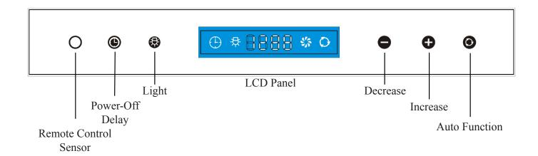
In addition to the remote control feature, this range hood is also equipped with a heat sensor that will self-calibrate in 5 seconds when the range hood is first electrically activated and beeps when self-calibration is done. To conserve energy, the LCD panel will turn off automatically after 5 seconds of inactivity.
