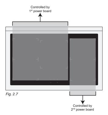
Should the cooking zones of one power board require more than the maximum total power, the last selected power level has priority and the power of the other cooking zone(s) is automatically reduced to the remaining power available (or switched off if there is not enough power available).
