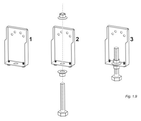
1. Thread the bolt through the adjustable bracket and fix in place using the two supplied nuts. Ensure the nuts are well tightened.
