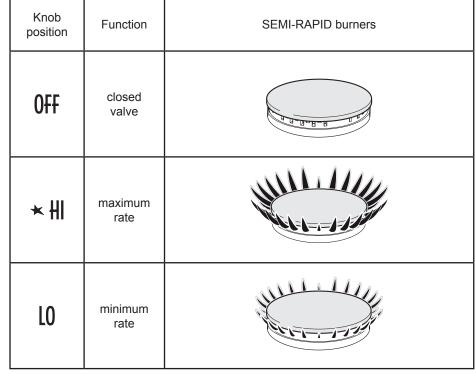
The maximum aperture position permits rapid boiling of liquids, whereas the minimum aperture position allows simmer warming of food or maintaining boiling conditions of liquids.
