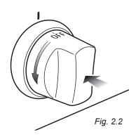
N.B. When the range is not being used, set the gas knobs to their **Off** positions and also close the gas shut-off valve placed on the main gas supply line.
