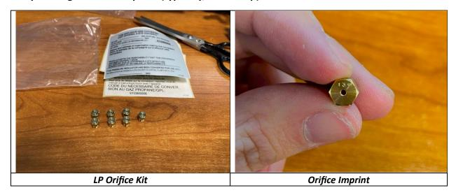
It is now time to swap orifices from each burner. Remove burner grates, caps, and heads.
