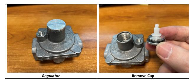
Gently unscrew the gas regulation screw. Once removed, flip and screw in as shown below.
